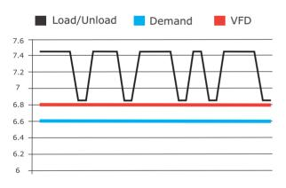
Typical Pressure pattern using a standard compressor and a compressor with VFD
